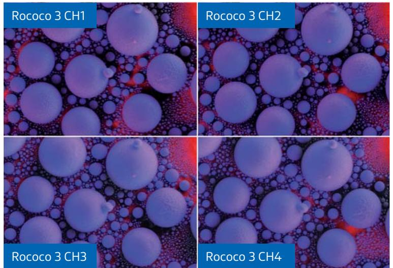
Particle analysis of a fly ash sample with the Rococo 3 detector.
